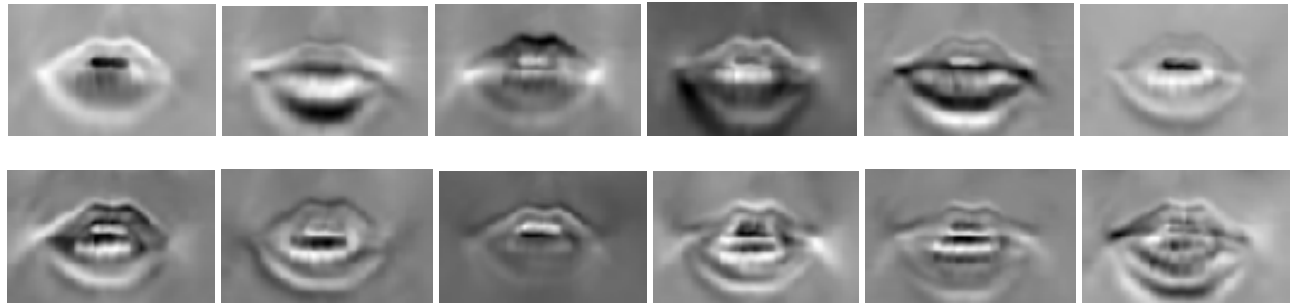
Figure 2.28. Principal Component Analysis. These are the first twelve principal components of the database of 200K normalized mouths. Only the luminance channel is used for the analysis. The resolution of the normalized mouths is 86x54 pixels.
