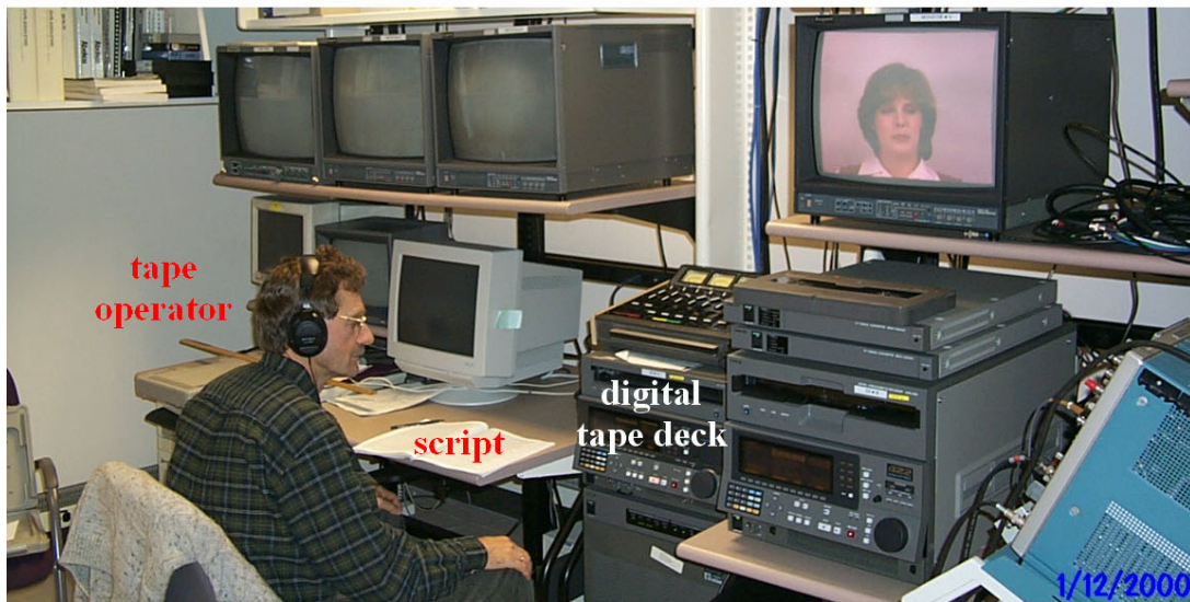
Figure 2.14. Snapshots of the recording session. The talent sits in a separate 'silent' room and reads from a teleprompter. A 3CCD camera transmits a RGB component signal to the recording room, which is recorded uncompressed digitally onto D1 tapes. The audio is also recorded digitally from a directional microphone onto the same tape.
