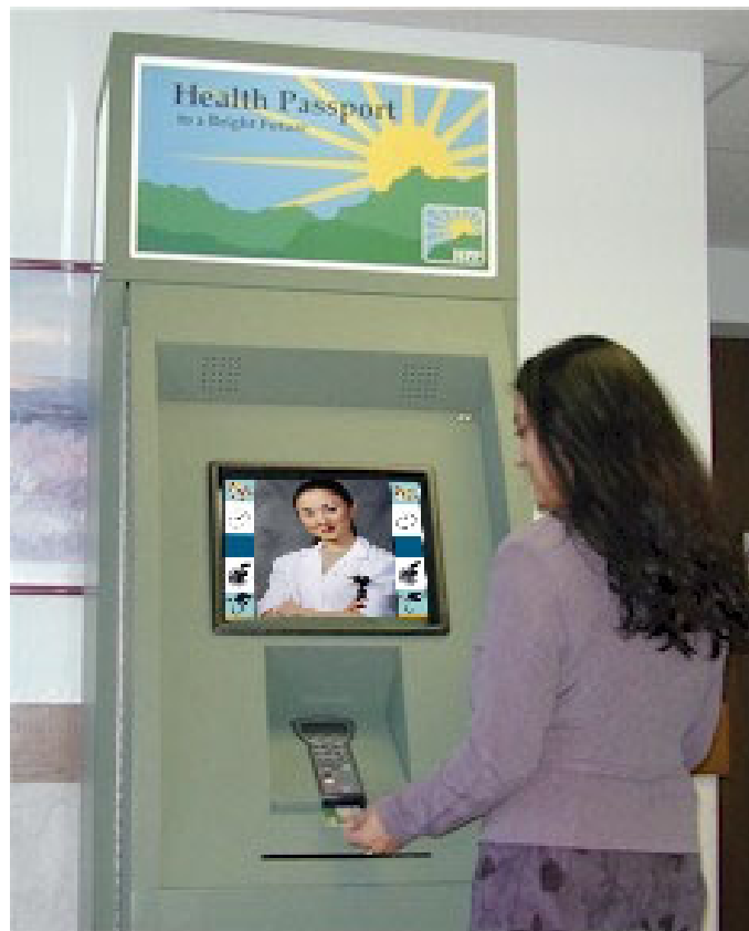
Figure 1.3. Mock-up of an automated healthcare kiosk. The user inserts her health card which contains her medical history and the talking head interacts with her to get the symptoms and issue the diagnostic. Trust in the system is much improved by the presence of the virtual doctor.
