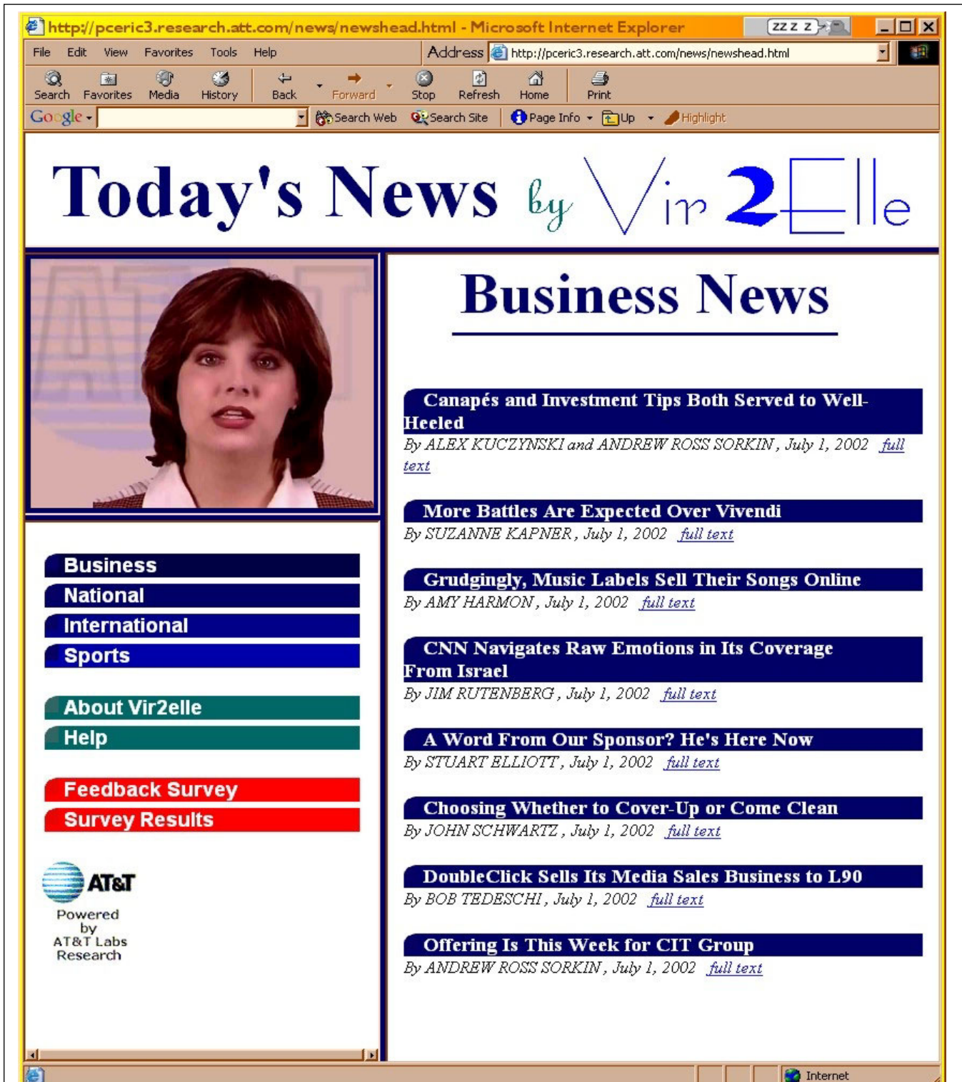
Figure 3.25. Screenshot of the Automatic Newscaster application. The web site is organized using page frames. On the left side of the screen our talking-head is speaking a summary of the headlines, while on the right side of the screen, the user can click on any headline and have the talking-head directly skip to it or alternatively access the full text for reading. The talking-head animation is generated entirely automatically from the textual content downloaded from the Internet.
