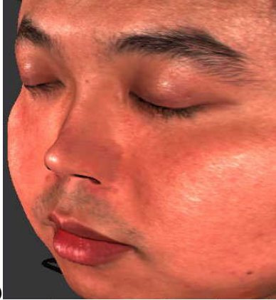
Figure 2.13. Examples of CyberWare scans at different stages. The range data (a), the texture (b) flattened out using cylindrical coordinates. Bitmap (c) shows a 3D view of the scan, (d) shows the same view with texture applied. In (e) a detail is shown with shading.
